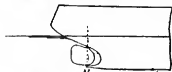
FIG. 71.—H.M.S. "Powerful." H.M.S. "Diadem" similar. in conjunction with a considerable cut-up at the stern in order to obtain increased manœuvring capacity (fig. 73). Recent second-class cruisers have rudders of the type shown in fig. 69.
